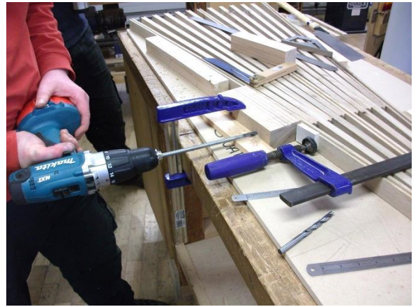
Image 37 Drilling hole for threaded bar
