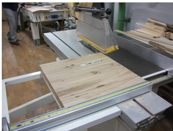
Image 46 Trimming rough edges of seat
