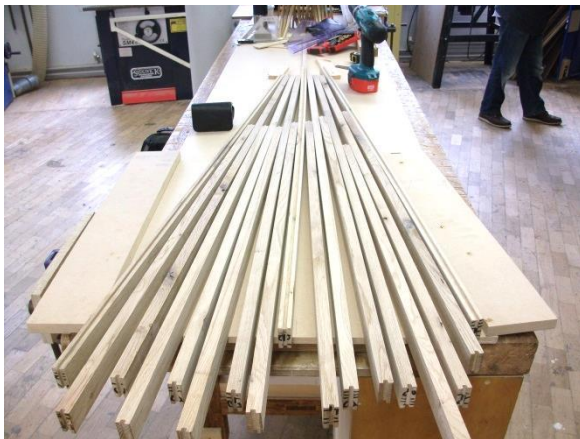
Image 34 Backrest laths arranged on jig board
