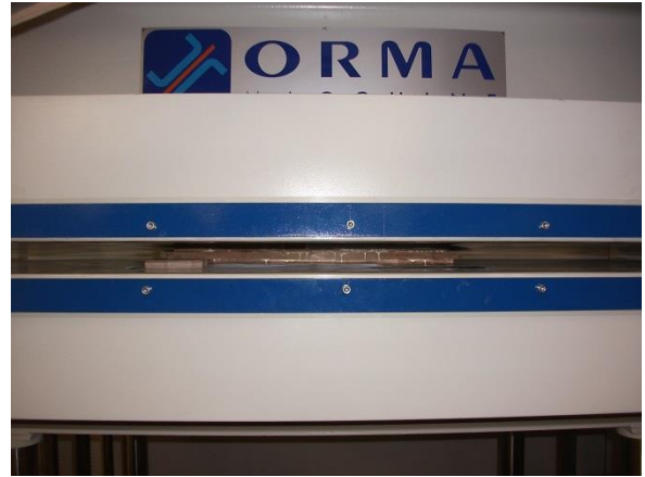
Image 31 clamping seat layer in heated press
