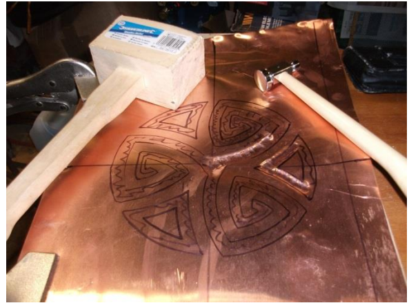
Image 85 Hammering design into copper with backing former
