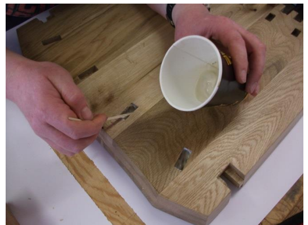
Image 71 Applying glue to leg mortises
