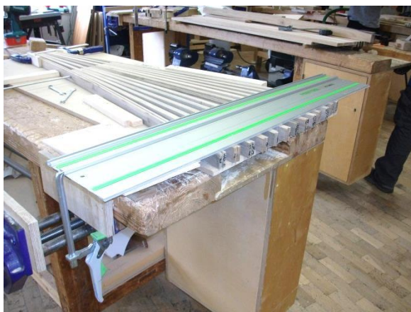
Image 40 Clamp on track for track saw
