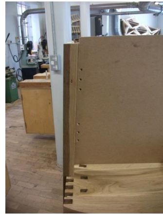
Image 69 laths fitted and glued to 5 deg. angle
