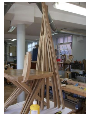
Image 75 Remaining lath fed on to threaded bar
