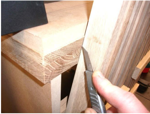
Image 48 Scribing lath positions to seat back Image 49 squaring these scribes to seat face
