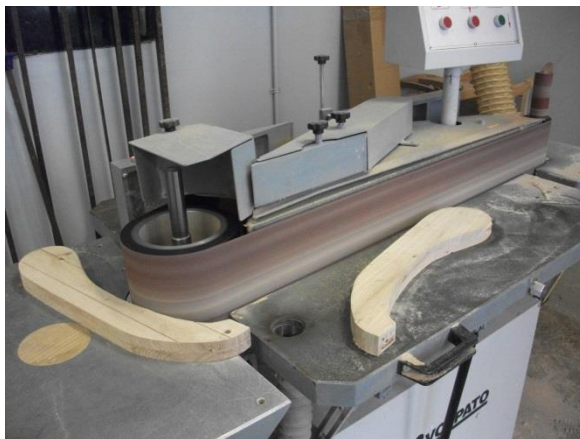
Image 58 Sanding cut out arms to shape
