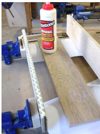
Image 28 Applying glue for rubbed joint
