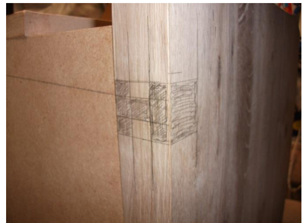
Image 59 Marking out of seat for arm post joint
