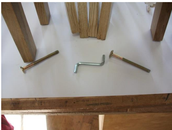
Image 76 Cot bolts ready for fitting
