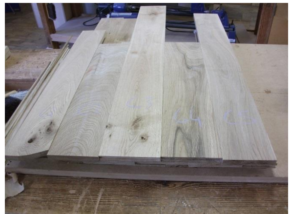
Image 27 Arranging layer of seat boards
