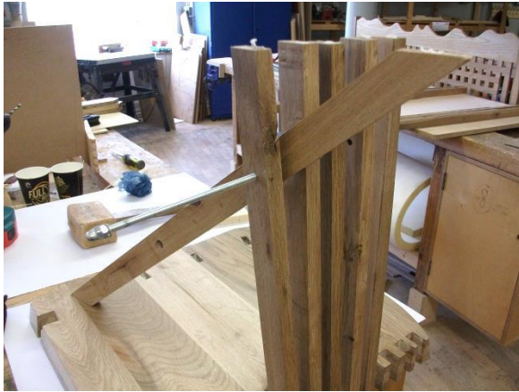
Image 72 Fitting threaded bar through legs and backrest
