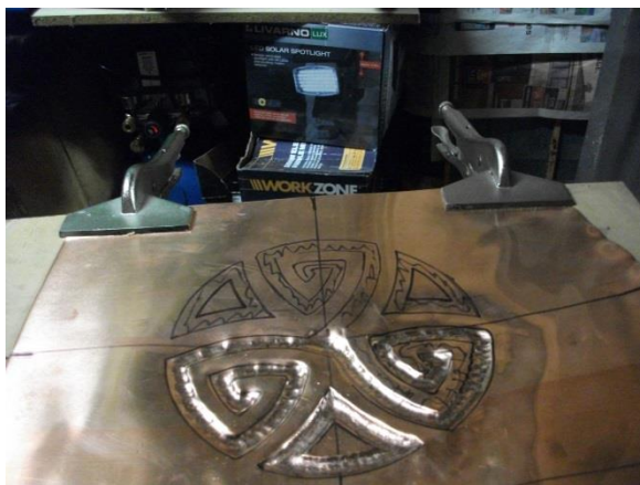
Image 82 copper clamped to design former
