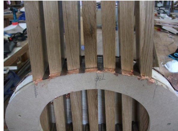
Image 85 Hammering design into copper with backing former
