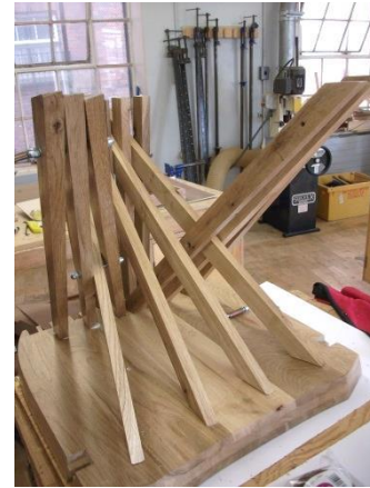
Image 73 Threaded bar fitted at leg crossing
