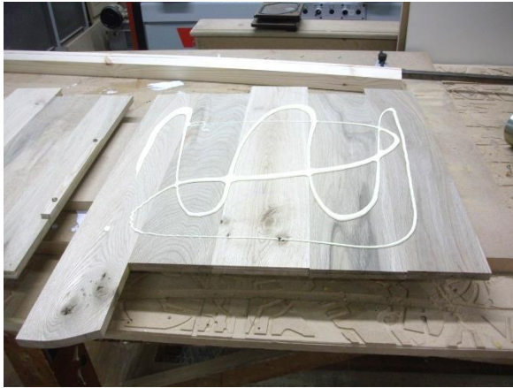
Image 30 Applying glue between seat layers
