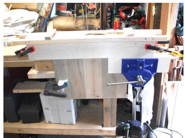
Image 51 Clamping seat and router jig in vice
