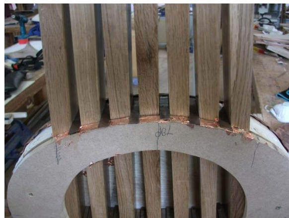
Image 85 Hammering design into copper with backing former
