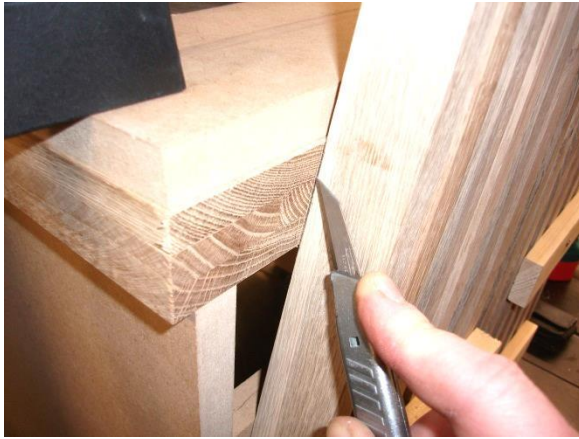
Image 48 Scribing lath positions to seat back Image 49 squaring these scribes to seat face
