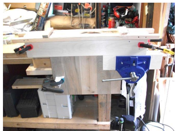
Image 51 Clamping seat and router jig in vice
