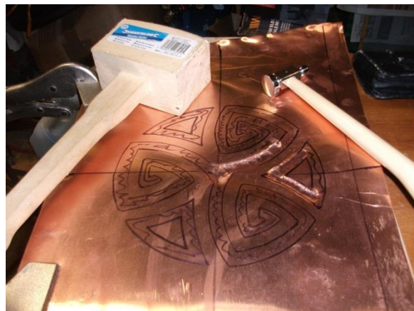
Image 85 Hammering design into copper with backing former
