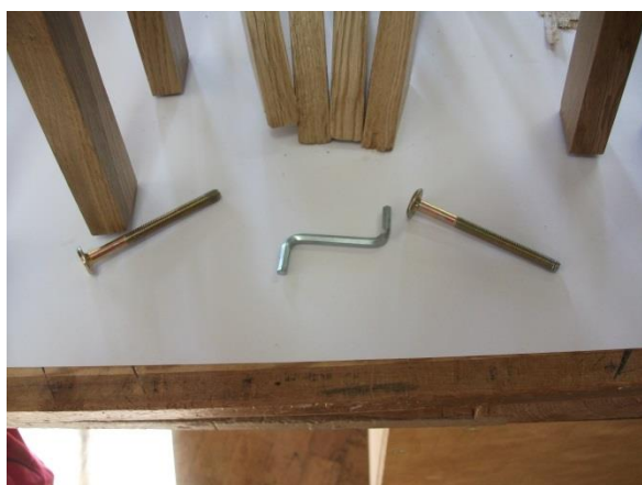
Image 76 Cot bolts ready for fitting
