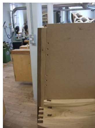
Image 69 laths fitted and glued to 5 deg. angle
