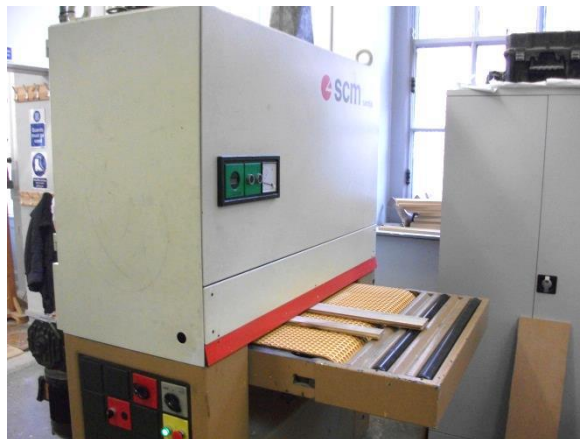
Image 25 Sanding off pre finished surface
