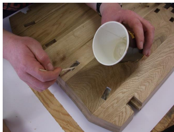
Image 71 Applying glue to leg mortises
