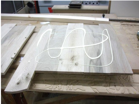
Image 30 Applying glue between seat layers
