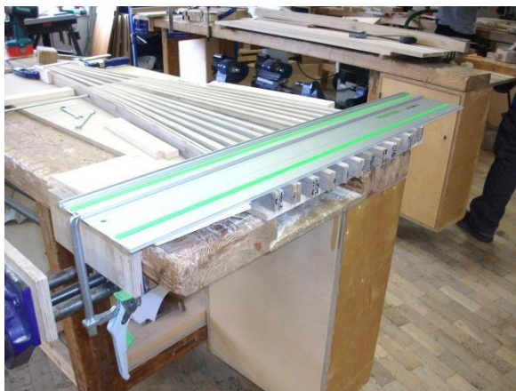
Image 40 Clamp on track for track saw
