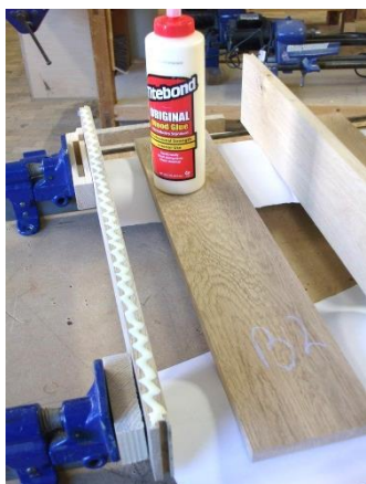
Image 28 Applying glue for rubbed joint
