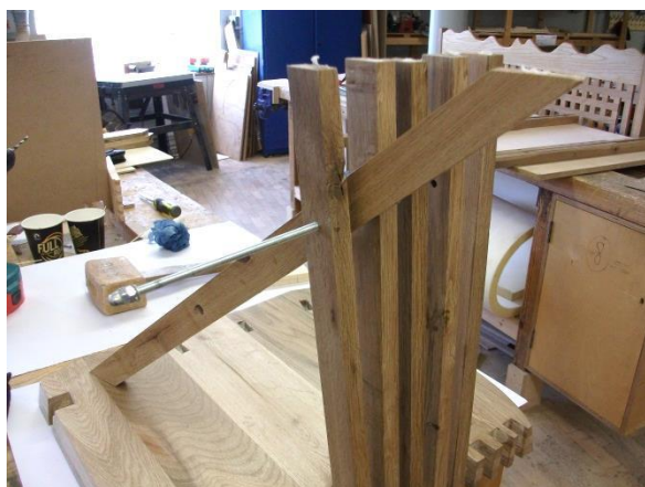
Image 72 Fitting threaded bar through legs and backrest
