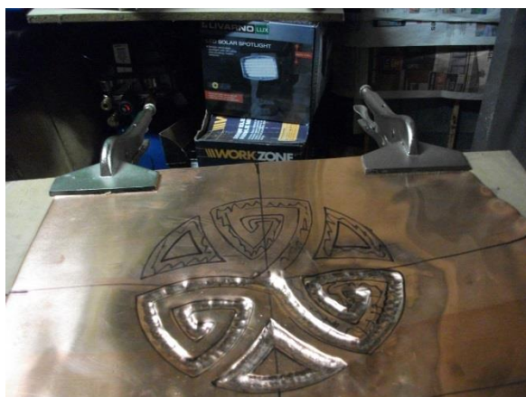
Image 82 copper clamped to design former
