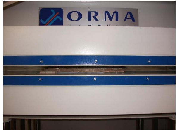
Image 31 clamping seat layer in heated press
