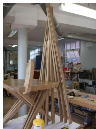
Image 75 Remaining lath fed on to threaded bar
