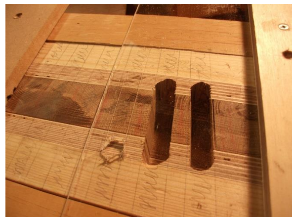
Image 53 Marking jig for router cutter
