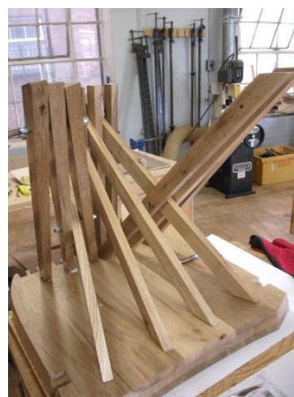
Image 73 Threaded bar fitted at leg crossing
