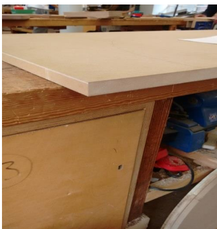
Fig. 54 25mm M.D.F. for formers.
