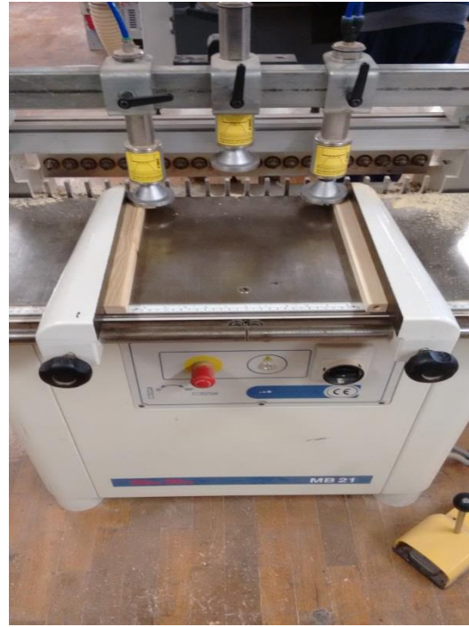
Fig. 68 Drilling on Dowel Machine.
