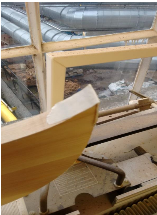
Fig. 45 Chipped piece glued and taped.
