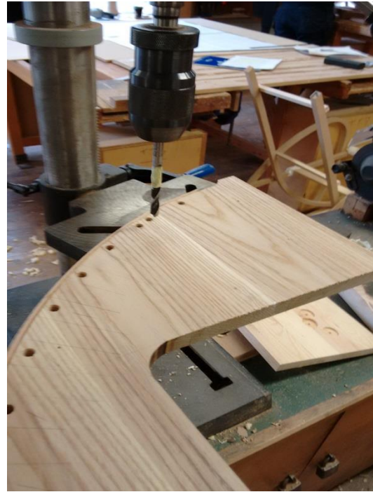
Fig. 76 Drilling Seat on the Drill Press.
