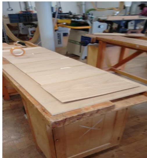
Fig. 62 Veneer strips taped together.
