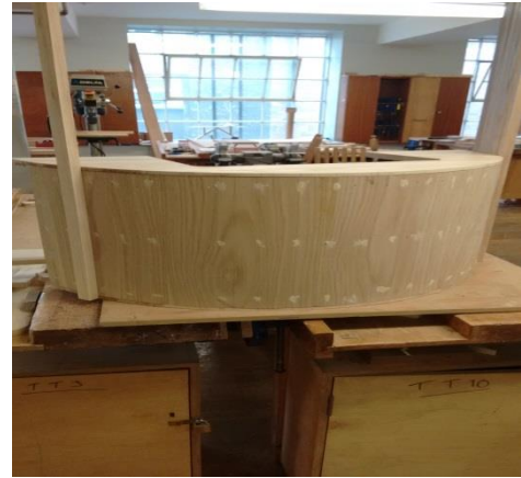
Fig.80 Pin Holes Filled.
