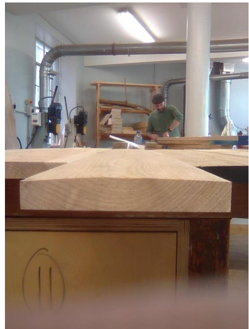
Fig. 25 3 edges planed on the timber.
