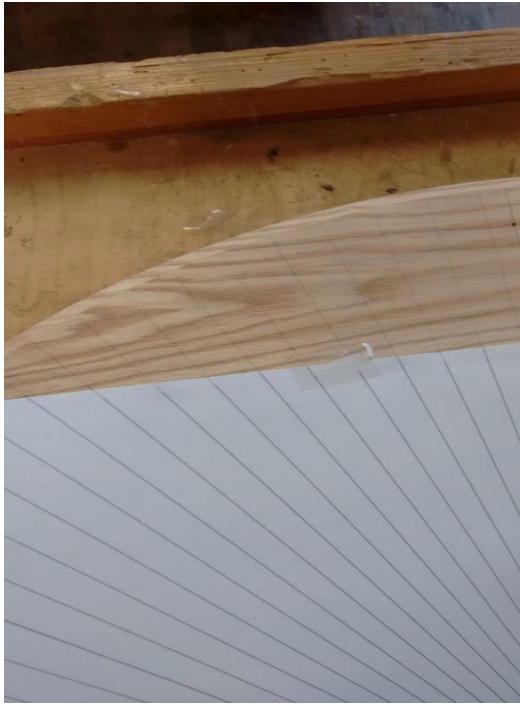
Fig. 67 Marking Upright positions.
