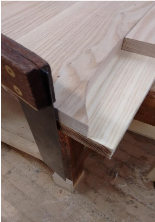
Fig. 49 Marking the 50mm line.
