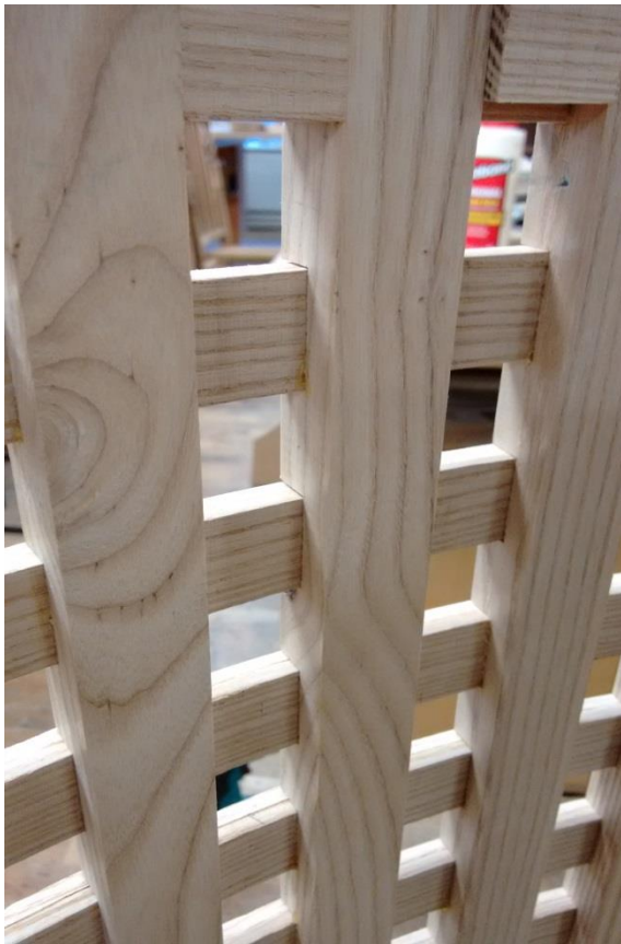
Fig. 98 Curves prior to squares being fitted.
