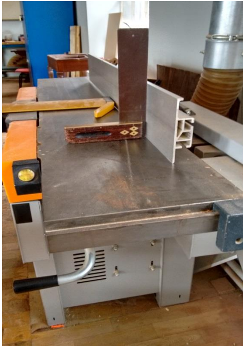
Fig. 22 Squaring the fence on the Planer.
