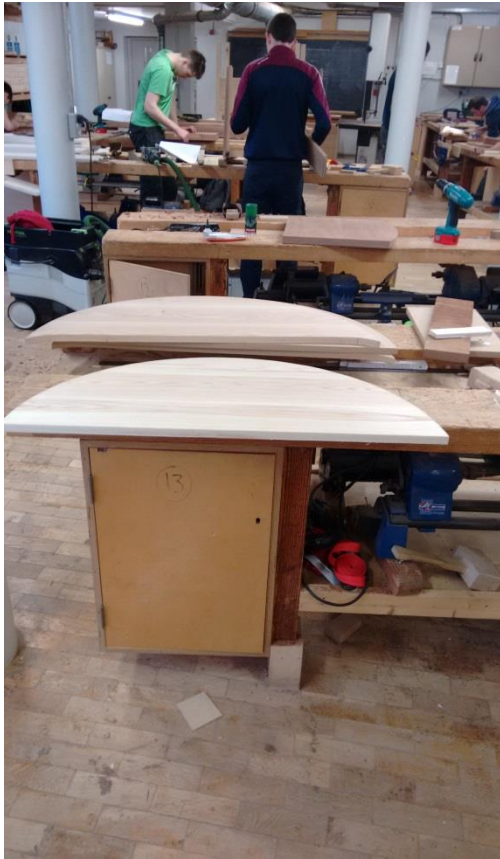
Fig. 47 Seat plank shaped.
