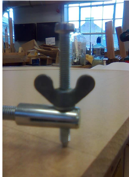
Fig. 36 Metal wind-on point for threaded bar.
