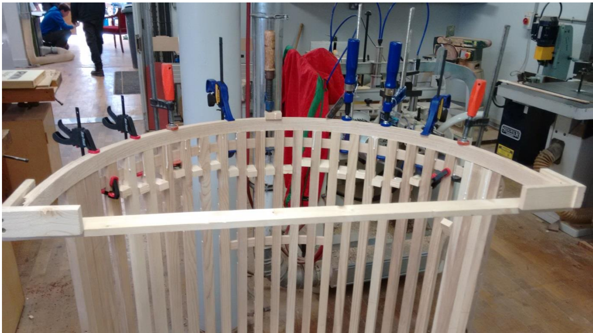
Fig. 88 Top Rail Cramped into position with bracing still attached.
