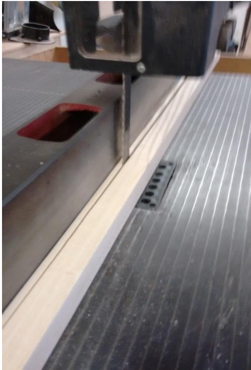
Fig. 56 Ripping 5mm strips on the band-saw.
