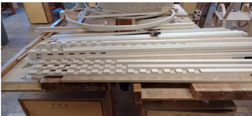
Fig. 81 Notches Cut Out of Uprights.
