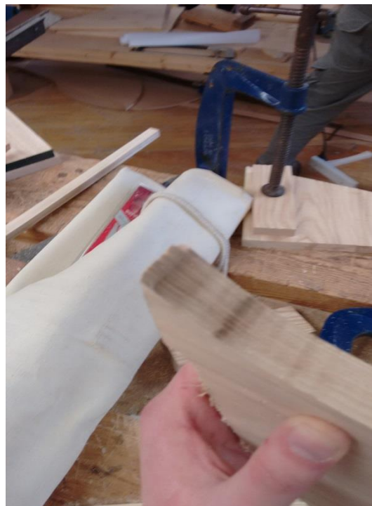
Fig. 46 Chipped piece repaired.
