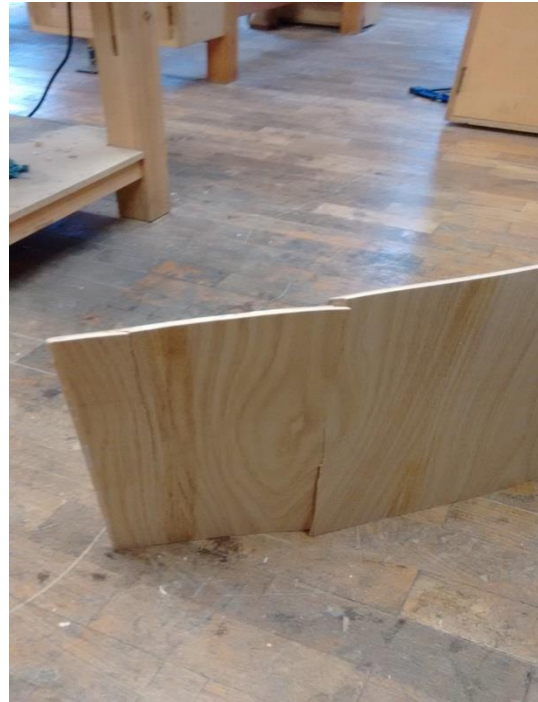
Fig.66 Split in veneered flexi-ply.
