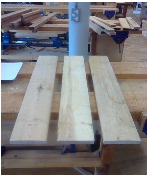
Fig. 20 Rough lengths of material for the base.
