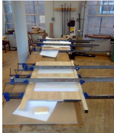
Fig. 29 2 groups of 3 lengths cramped.
