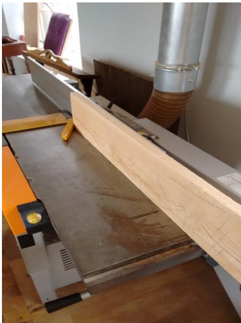
Fig. 24 Planing narrow edge off the fence.
