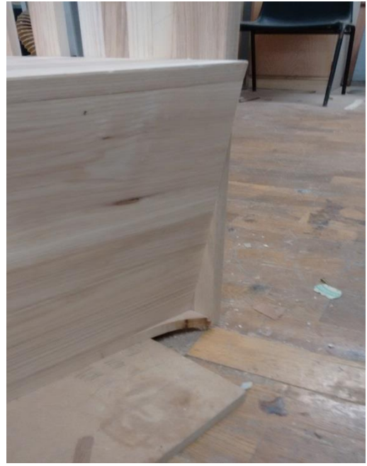
Fig. 96 Sloped front fitted to base.
