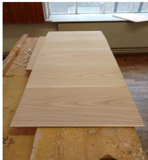
Fig. 64 Veneer trimmed off flexi-ply.
