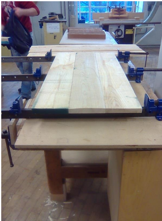
Fig. 26 3 Lengths laid out on the sash cramps.
