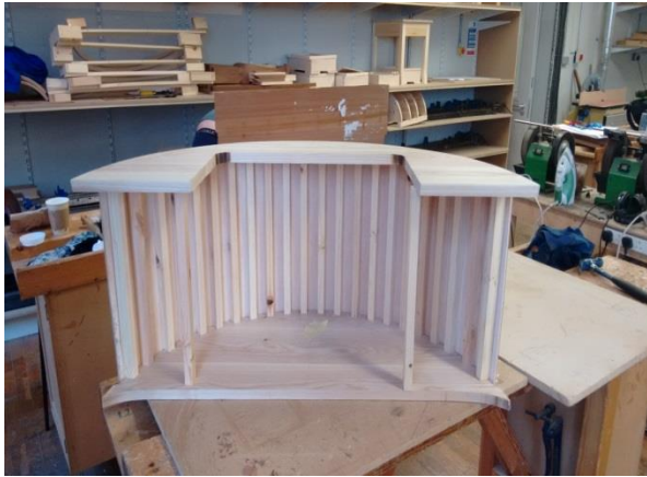
Fig. 79 Base After Being Cramped.
