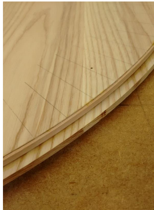
Fig.70 Strips glued in place.
