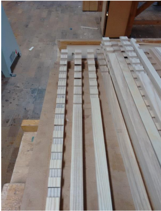
Fig. 82 Notches Out of Uprights.
