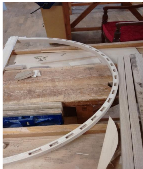
Fig. 85 Top rail after Mortises.
