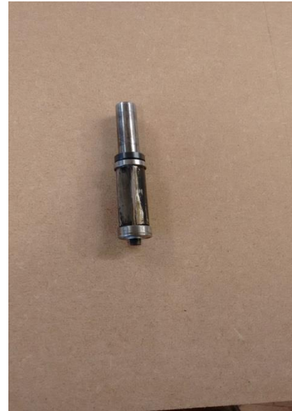
Fig. 42 Router trimming bit.
