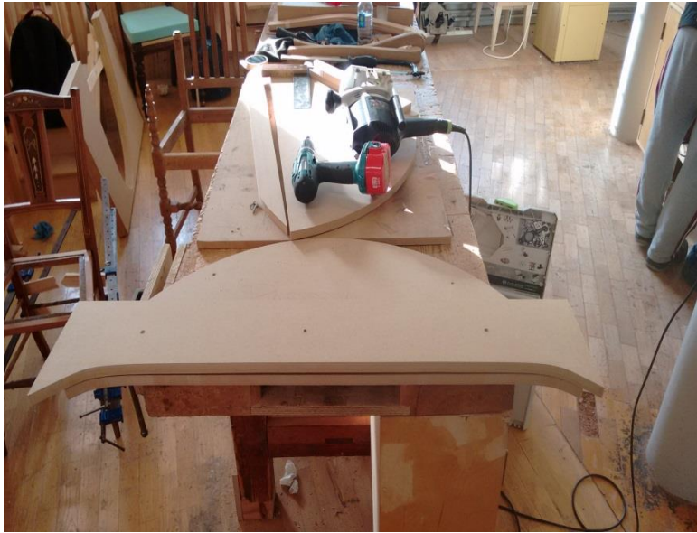
Fig.41 Full base bottom curve template fixed in place.
