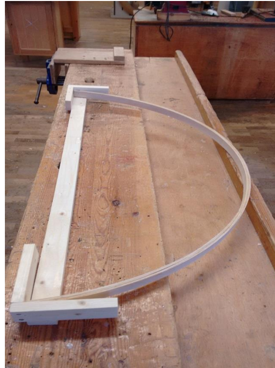
Fig. 60 Braced to maintain curve.
