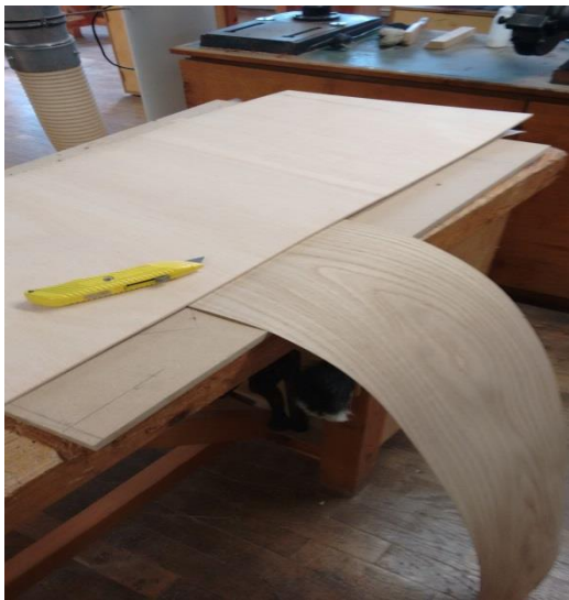
Fig. 61 Cutting out strips of oak veneer.
