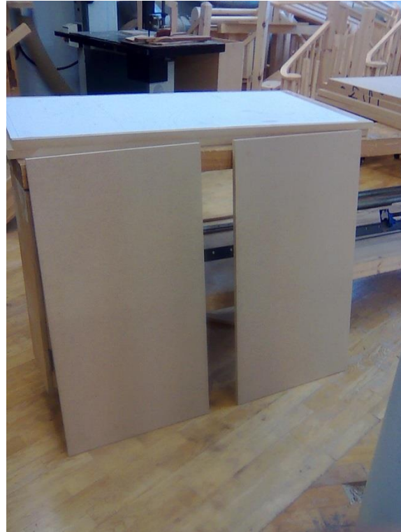
Fig. 34 Two M.D.F. pieces ready for routing.
