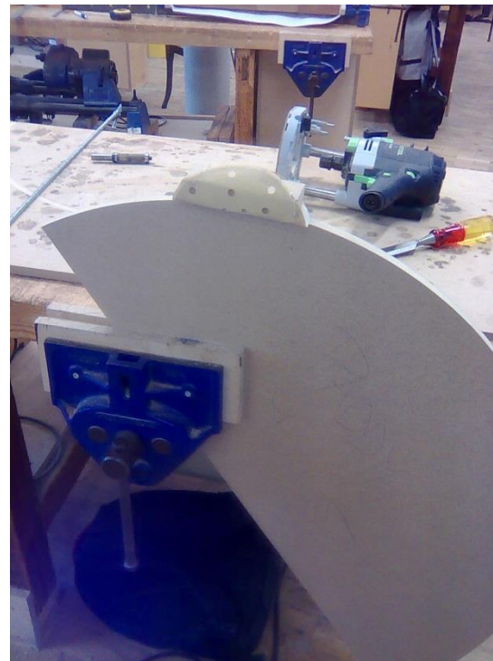
Fig. 38 Sanding down the template edge.
