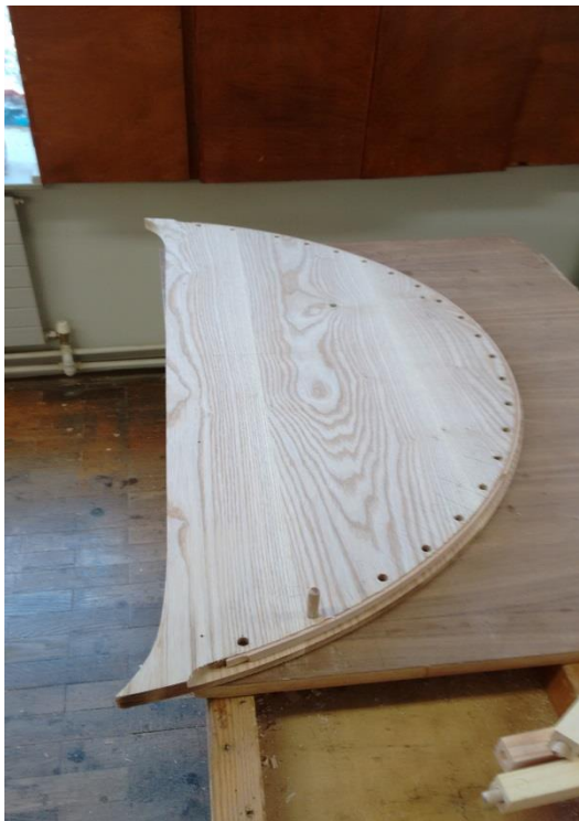
Fig. 77 Base Bottom Ready to be Cramped.
