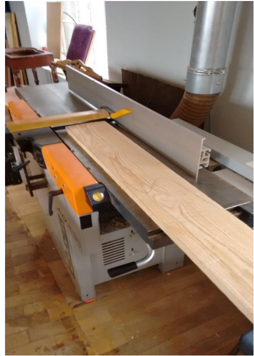
Fig. 23 Planing timber on the wide edge.
