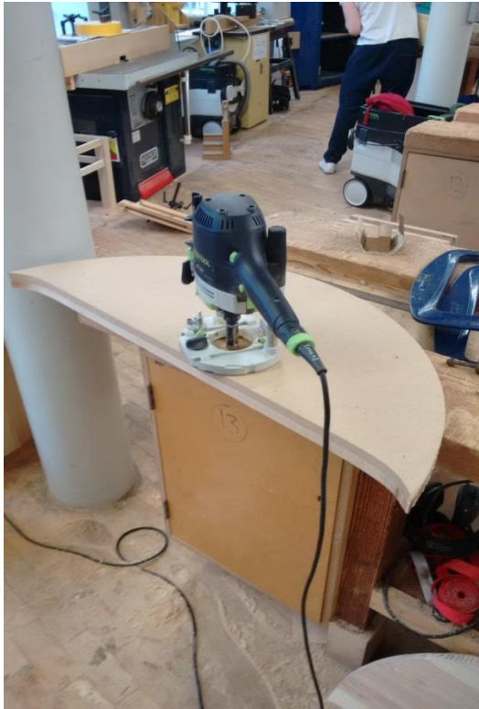
Fig. 43 Trimming around base bottom temp.
