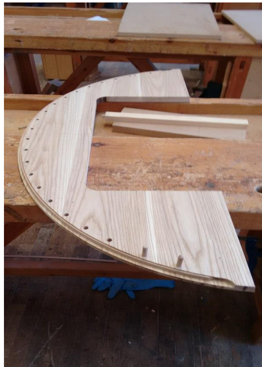
Fig. 78 Seat Ready to be Cramped.
