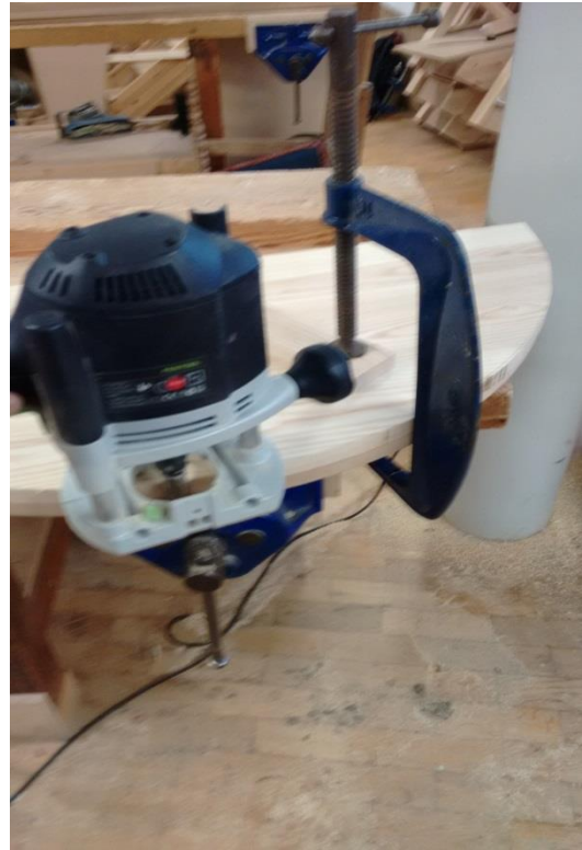
Fig. 44 Trimming around seat template.
