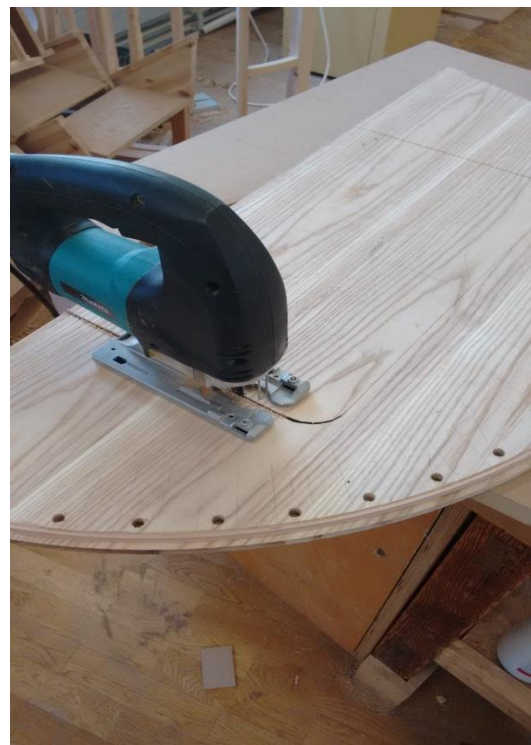
Fig. 74 Cutting out the Flap with the Jig-Saw.
