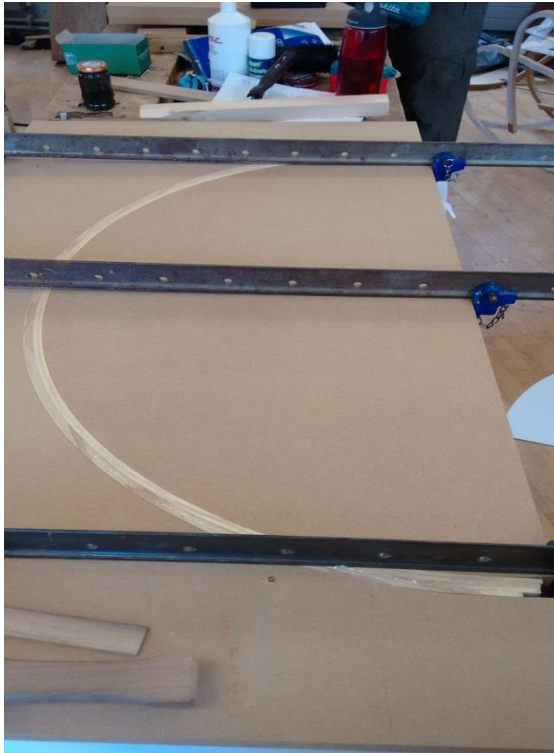
Fig. 59 Inner and outer strips cramped up.
