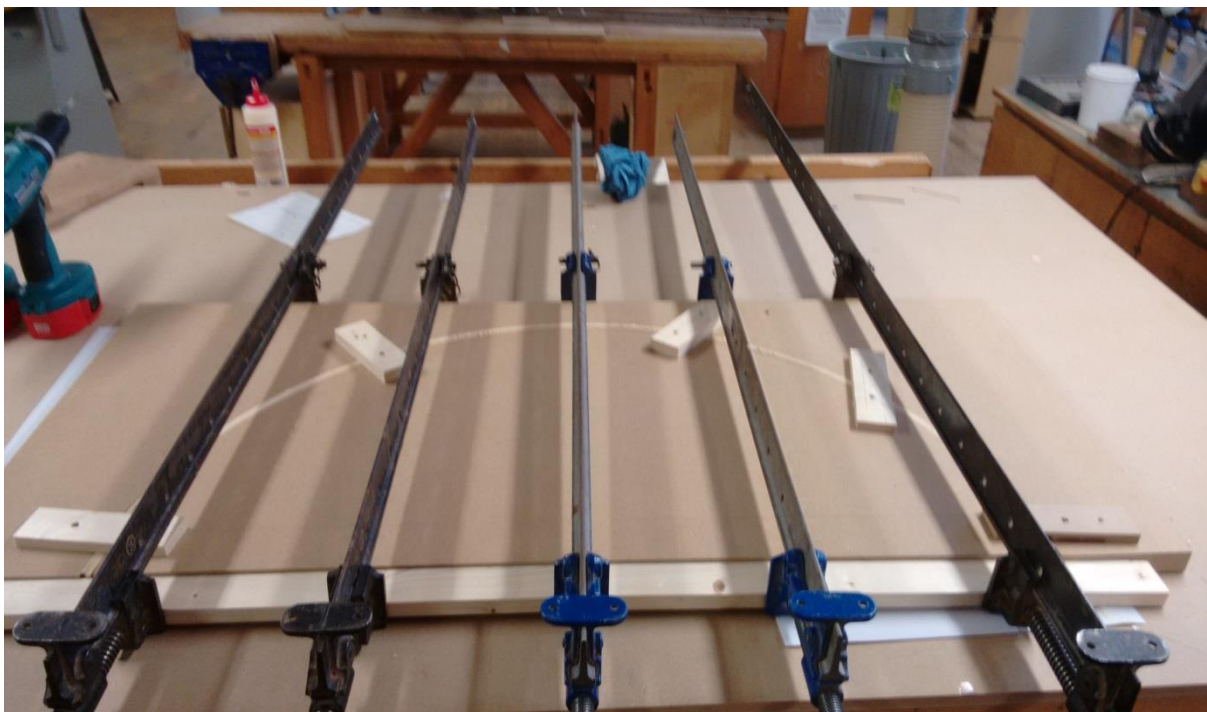
Fig. 58 Two inner 10mm curve strips in formers.
