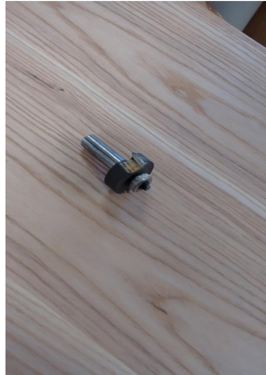
Fig. 50 10mm wheeled rebate bit.
