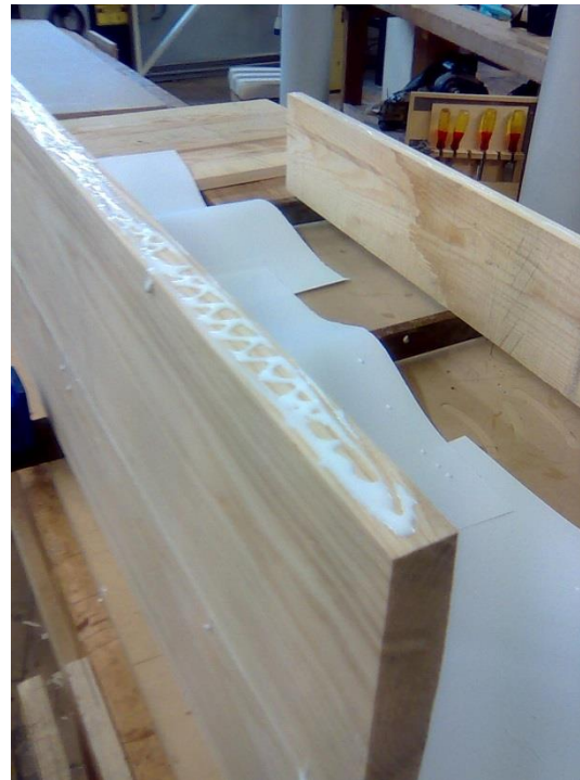
Fig. 27 Glue applied to narrow edge.
