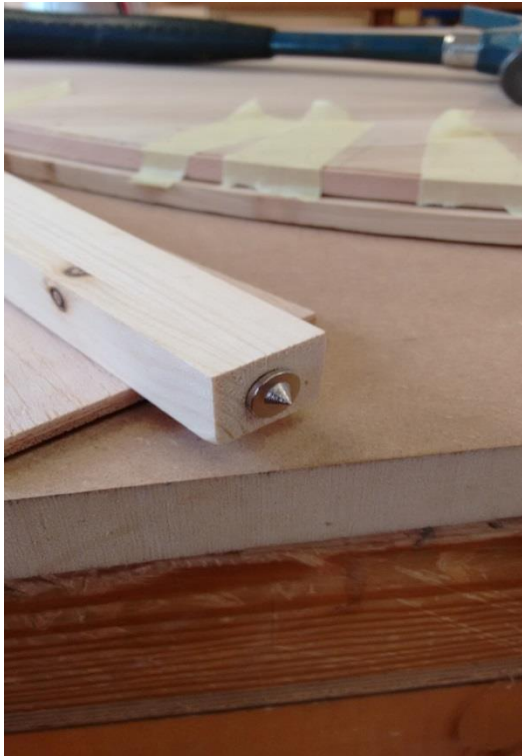
Fig. 71 Dowel Marker in Upright.
