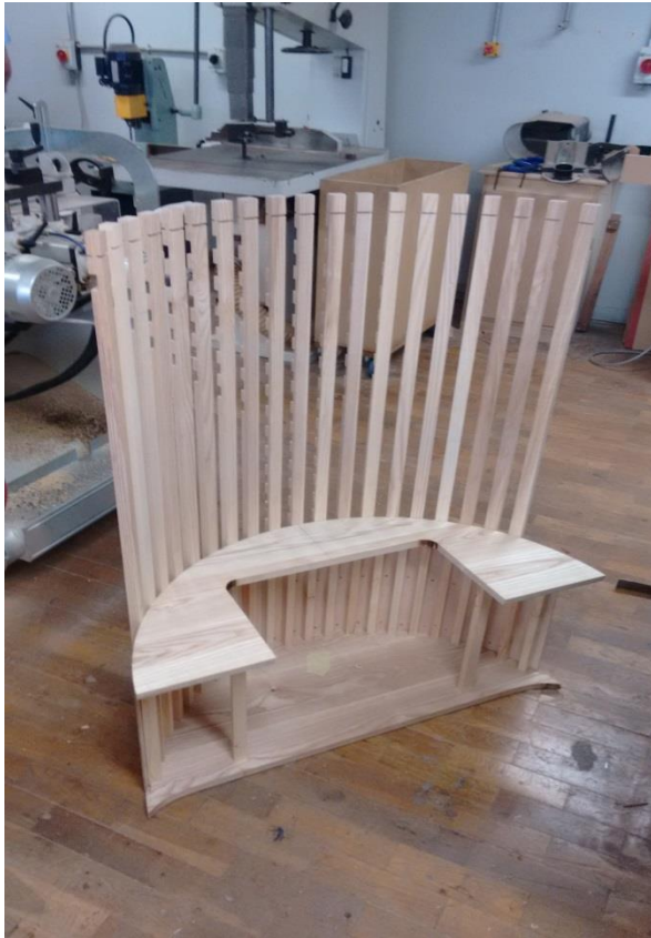
Fig. 86 Uprights fixed in place.
